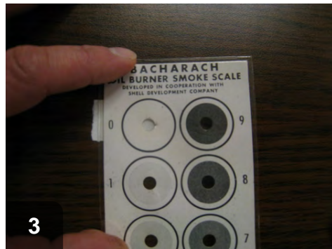
3 Compare level of soot deposit against smoke chart. A rating of 0 is ideal
