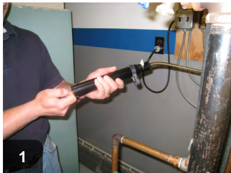
1 Place filter paper in testing pump and draw air through paper
