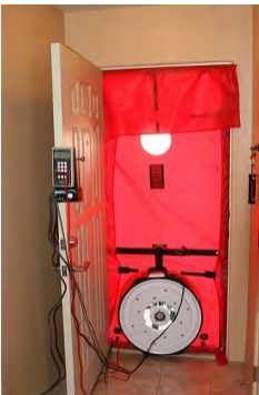
Set up blower door and depressurize bonus room to -50pa wrt outside
