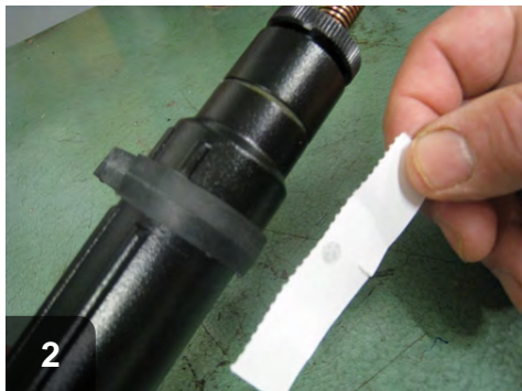
2 Remove paper and verify draw was successful by checking for soot
