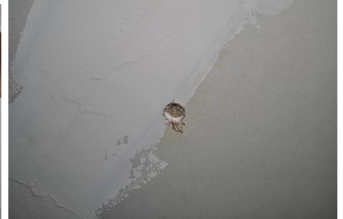
Cut small test holes in cavities to verify specified density has been met
