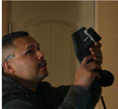
Inspect for voids and low density areas
