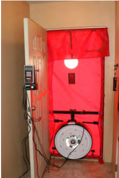
Depressurize house (if safe) to -50pa wrt outside
