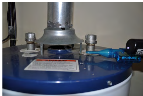
Complete spillage test using chemical smoke pencil
