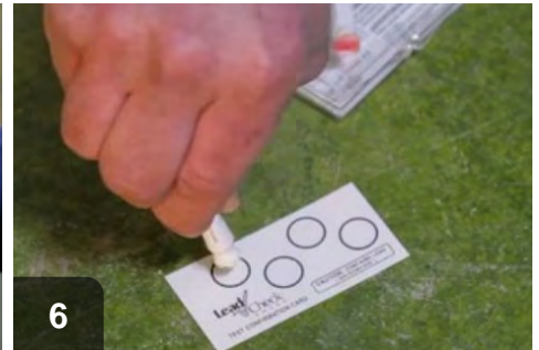
6 If negative, verify validity of test with provided calibration card
