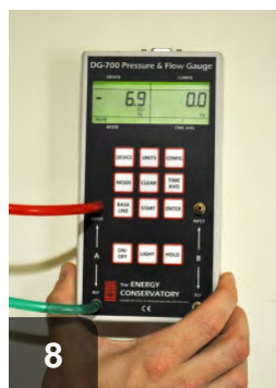
8 Manometer reading should not be more negative than -3pa
