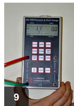
9 If reading is within allowable limit, all is well
